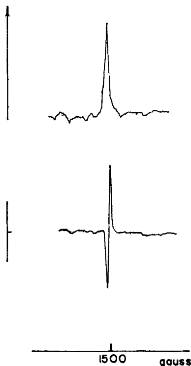
Figure 6. The \Delta m = \pm 2 transition of naphthalene- d_8 in durene. The modulation depth of the MODOR line is approximately 0.3%.
